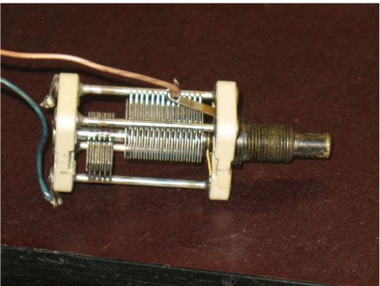
Now that the assembly is out, let's remove the variable capacitor from it's cover. In order to do that, the gear will need to be removed first. I found this very beneficial post by Roger in the 'Pearls'
