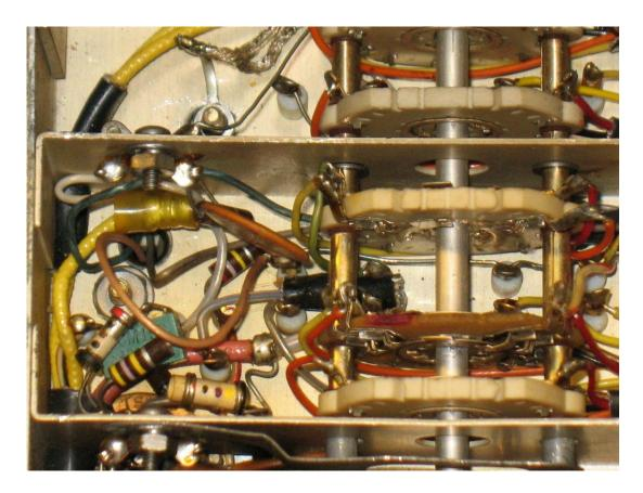
The following two pictures show where these two wires are connected, so you can put them back in the right place. The other end of the brown wire is connected to the rotor on the capacitor while this end is connected to the AGC line. The blue wire is connected to the switch contact.
