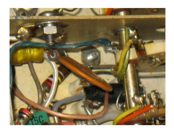
Once the two wires and two nuts are removed, the capacitor and cover assembly can be removed a few inches so that you can disconnect the gray wire from the capacitor. If it's too short, also disconnect it from the switch. At this point, you should be able to remove the assembly shown here.
