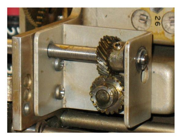
Now with both shafts removed, it's easier to remove the two short screws holding the 1 3/4" by 1 3/8" U shaped frame onto the rear gear frame. These are shown on the left side of the above picture between the two shafts that were removed. The next picture shows the two screws removed.
