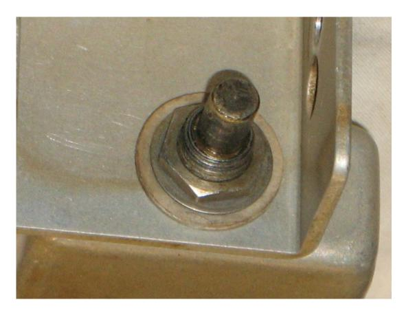
The nut needs to be firmly tight, but not so tight that it will damage the insulators. The capacitor cover must be oriented correctly to the bracket so that the screws go into the holes in the chassis like in this next picture:
