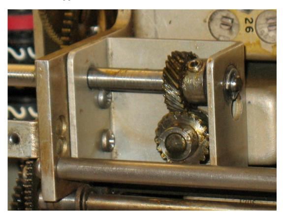
When I removed the RF deck, I took it out with the 2<sup>nd</sup> crystal oscillator attached, as it's much easier that way. Once the 'Ant Trim' shaft is removed, the next step would be to remove the 1/4" rod brace that is 5 5/8" long that is right on top of the capacitor drive gear (shown above). It's held in place with a screw on each end and are easy to remove. Next is a picture with the rod brace removed.
