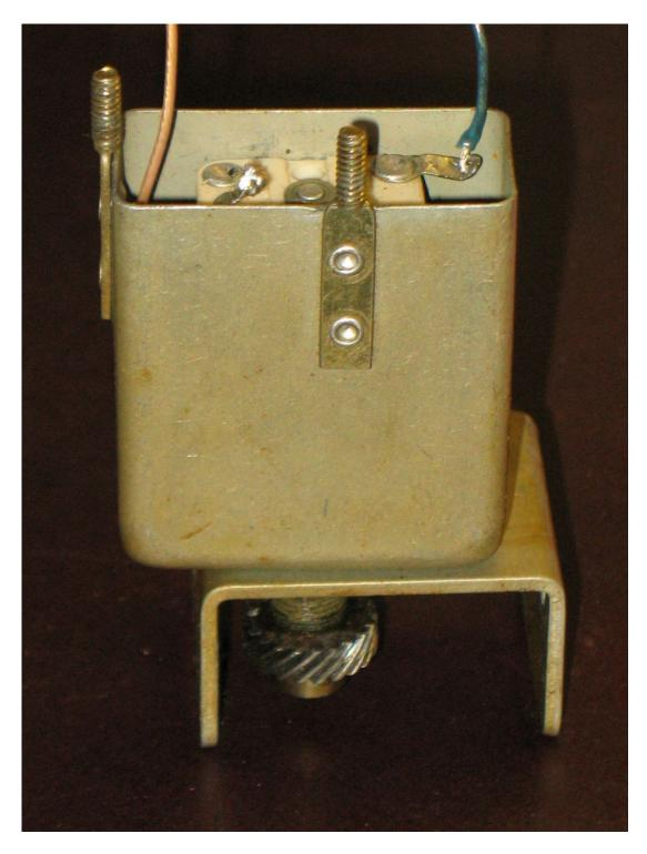
Before I put the gear on, I wanted to make one last check that the static problem (plate touching) and rotor grounding were fixed. Sure enough they are, so I proceeded to put the gear on.
