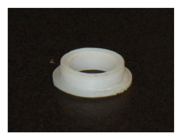
Although the spacing collar in the center on this one sticks up higher, this could still be used as it would space both the capacitor cover and the mounting bracket, and then just a flat insulating washer could be used on the top.
