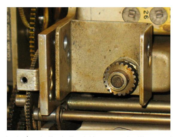
Since the 2<sup>nd</sup> crystal oscillator is still attached, it's not as easy as it could be to remove the top screw of the two, but a right angle phillips screw driver will help to loosen it up. Loosen the bottom one up the same way. I got this idea from part of this post in the Pearls RF Deck Mechanical:
